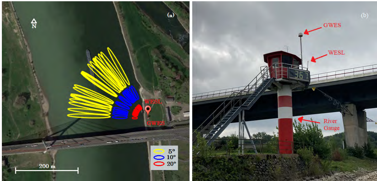
Figure 3.1.3.1: Test site GWES and WESL. (a) Location of the GNSS antenna GWES, the PRP WESL, and tide gauge in Rhine river, Wesel, Germany. Footprints of the reflected GPS signals are projected on a Google Earth image. Reflection zones corresponding to azimuth 260^{\circ} – 320^{\circ} and elevation 5^{\circ} and 15^{\circ} . (b) Both antennas were installed on top of a stilling well river structure. The tide gauge is in the same structure. Source: https://gnss-reflections.org/rzones
