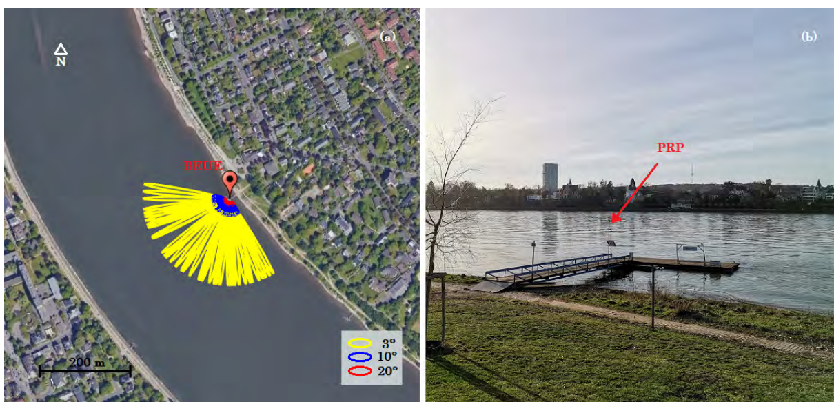
Figure 3.1.5.1: Test site BEUE. (a) Location of the PRP GPS antenna in Rhine river, Bonn-Beuel, Germany. Footprints of the reflected GPS signals are projected on a Google Earth image. Reflection zones corresponding to azimuth 140^\circ – 280^\circ and elevation 3^\circ and 20^\circ . (b) The PRP was installed on a pier. Source: https://gnss-reflections.org/rzones
