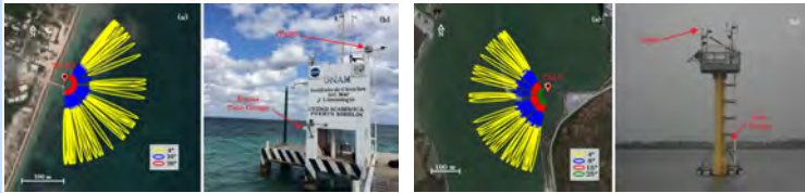
Fig. 1. Test site TGMX. (a) Mask, azimuth: 30°-190° and elevation angle: 4°-20°. (b) Location. Fig. 2. Test site CALC. (a) Mask, azimuth: 190°-340° and elevation angle 4°-25°. (b) Location.
