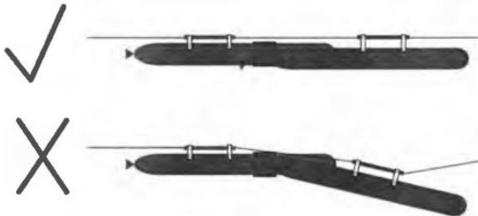
Figure 5. Balloons that are properly aligned (top) and misaligned (bottom).
