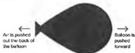
Figure 2. Newton's third law of motion for an inflated balloon.
