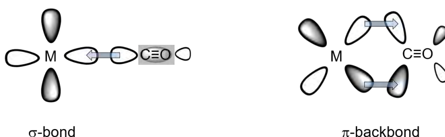
Figure 2.19 The \sigma and \pi bonding in metal carbonyls. The 2p\pi orbital of CO is antibonding, the backdonation of electron density to this orbital results in the weakening of the bond.
