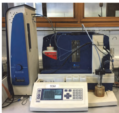
Figure 6. Equipment to perform pH-metric and pK_a experiments used in the determination of lipophilicity of compounds. (Sirius Analytical http://www.sirius-analytical.com )
